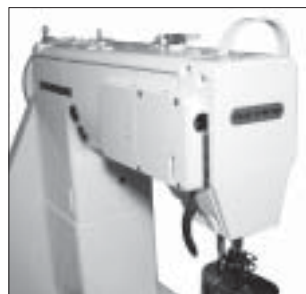
Open/close simplified face plate and upper feed mechanism
