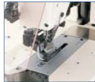
• This needle entry point can visually be checked. This permits easy positioning of buttonholes.
